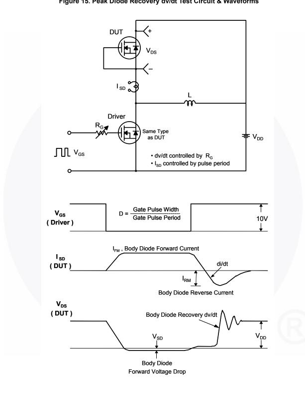
Figure 15. Peak Diode Recovery dv/dt Test Circuit & Waveforms
