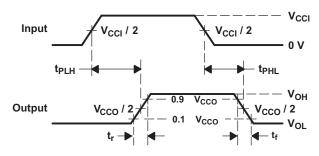
Figure 7. Propagation Delay Times
