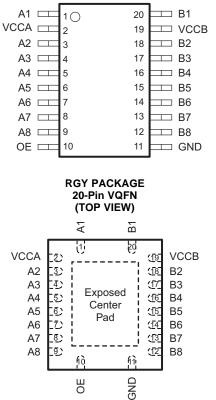
The exposed center pad, if used, must be connected as a secondary ground or left electrically open.
