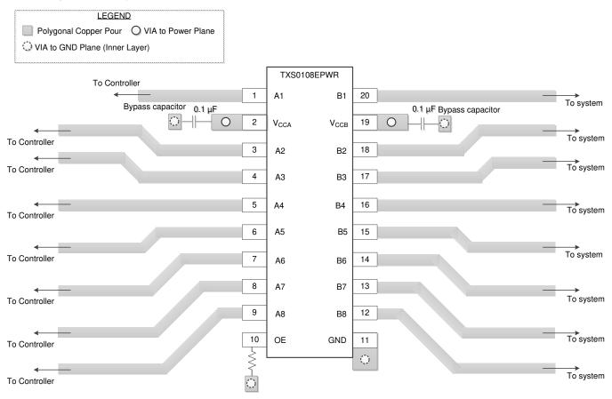
Keep OE low until  $V_{\text{CCA}}$  and  $V_{\text{CCB}}$  are powered up
