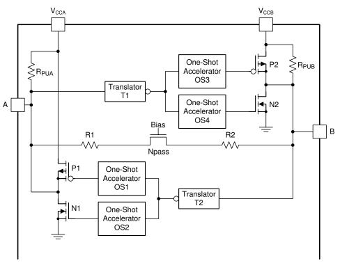
Figure 9. Architecture of a TXS0108E Cell
