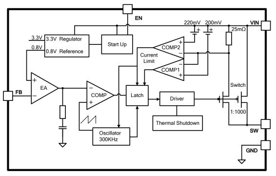
Figure 3. Function Block Diagram of XL4005
