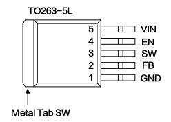
Figure 2. Pin Configuration of XL4005 (Top View)
